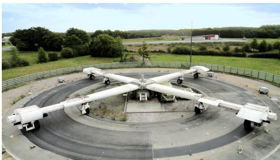
Figure 1: Accelerated pavement testing facility of IFSTTAR
