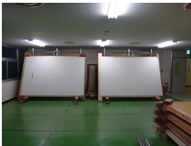
Figure 7: Wooden wall model specimens set in a laboratory room.
