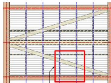
(a) Inner structure of the model under the regulation before 1995. Amplitude ( d=1.5\text{cm} )
