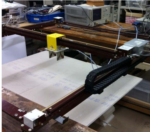
Figure 3: Setup of antenna son a antenna positioner
