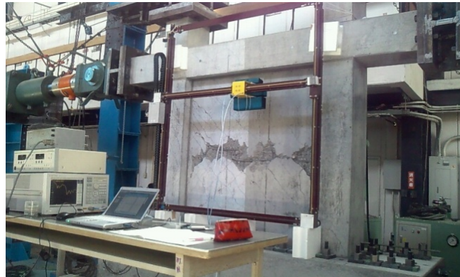
Figure 4: Concrete wall measurement setup.
