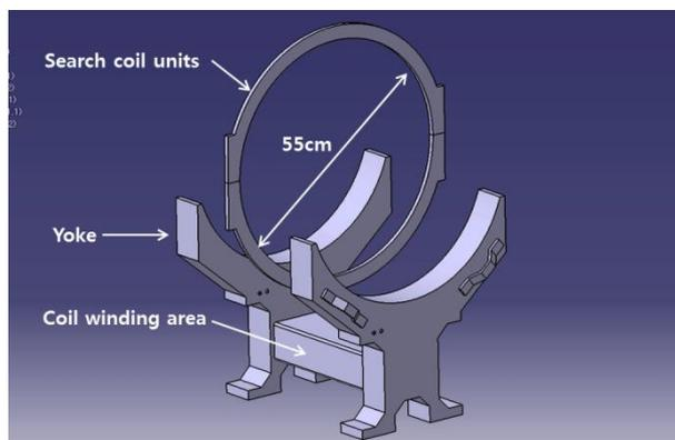
Figure 7: A detail drawing of the sensor head
