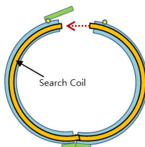
Figure 5: An open-able search coil sensor
