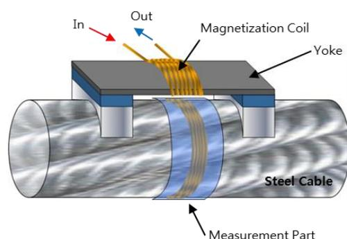
Figure 4: The concept of total flux sensor head
