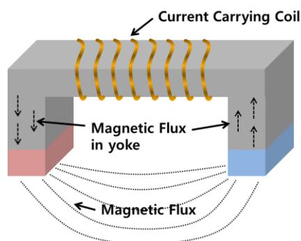
Figure 2: Yoke type electromagnet
