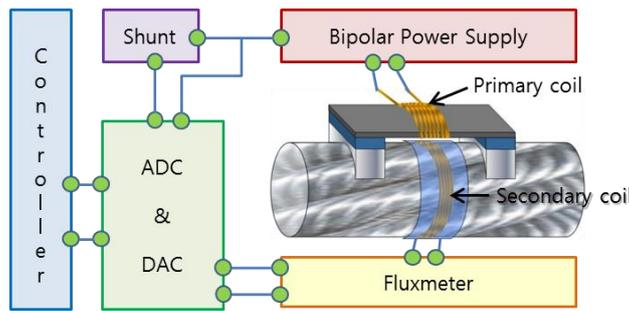
Figure 6: Schematic diagram of main cable NDT system
