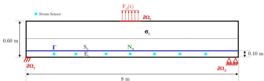
Figure 1 : Concrete beam with a horizontal steel bar - Beam instrumented with 7 strains sensors.
