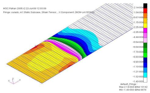
Figure 2: Residual strain in sensor layer for a debonding length of 25 mm.
