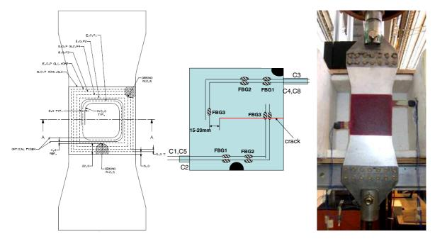
Figure 5: Left: Design of the Second Demonstrator. Middle: Bonding of the sensor mat and the repair patch on the second demonstrator. Right: second demonstrator in the fatigue test rig.
