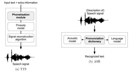
Figure 1: Architecture of (a) TTS and (b) ASR systems
