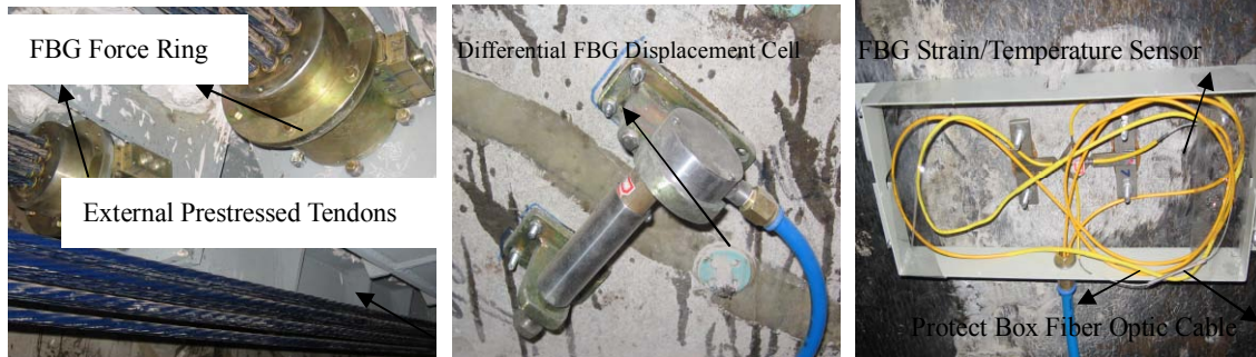
Fig.1 FBG force ring Fig.2 Differential FBG displacement cell Fig.3 FBG strain/temperature sensor
