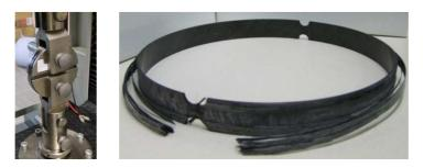
Figure 3: Experimental set-up (left) and NOL ring after failure (right)
