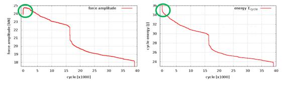
Figure 4: Typical low-cycle fatigue test expressed in force amplitude (left) and in energy (right) [6]
