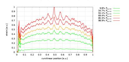
Figure 10: Strain profiles  $\Delta \varepsilon_{P_0 \to P_n}(s)$  during water-filling operation: baseline for structural monitoring regarding theoretical mechanical properties of the composite structure
