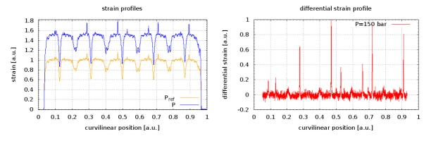
Figure 7: Differential strain profile  $\delta_K \Delta \varepsilon(s) - P_{ref} = 100 \text{ bar}$  and  $P = 150 \text{ bar} (P_0 = P_{atm})$  [6]
