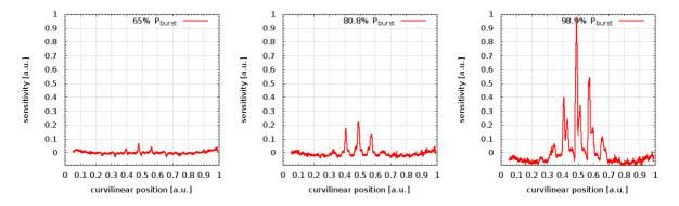
Figure 11: Differential strain sensitivity *vs.* pressure profile  $S_{(P_0, P_{ref}, P)}(s)$ : "instantaneous" strain deviations due to structural defects highlighted during the filling operation
