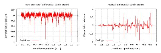
Figure 8: Differential strains with P = 40 bar (left) and residual differential strains with  $P = P_{atm}$  (right)
