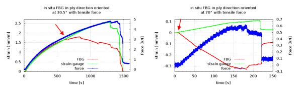
Figure 2: In situ (FBG) compared with surface (strain gauge) measurements during uniaxial tensile tests [6]
