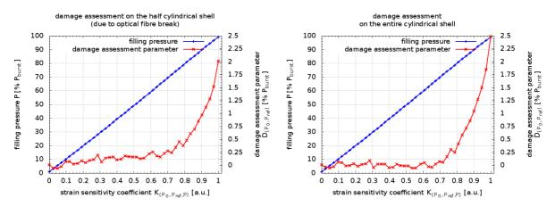
Figure 12: Pressure vessel damage assessment: evidences of critical damage starting at 70% burst pressure
