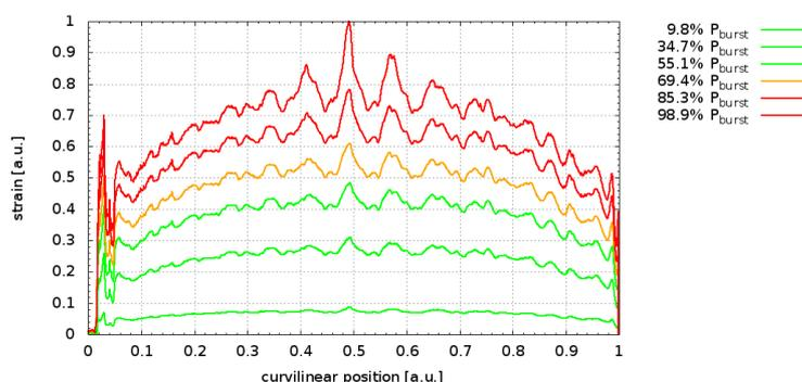
Figure 10: Strain profiles  $\Delta \epsilon_{P_0 \rightarrow P_n}(s)$  during water-filling operation: baseline for structural monitoring regarding theoretical mechanical properties of the composite structure
