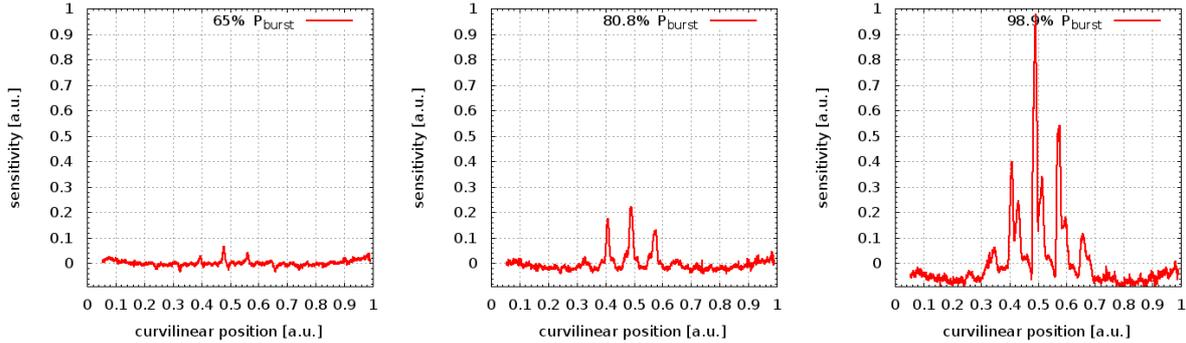
Figure 11: Differential strain sensitivity vs. pressure profile  $\mathcal{S}_{(P_0, P_{ref}, P)}(s)$ : “instantaneous” strain deviations due to structural defects highlighted during the filling operation
