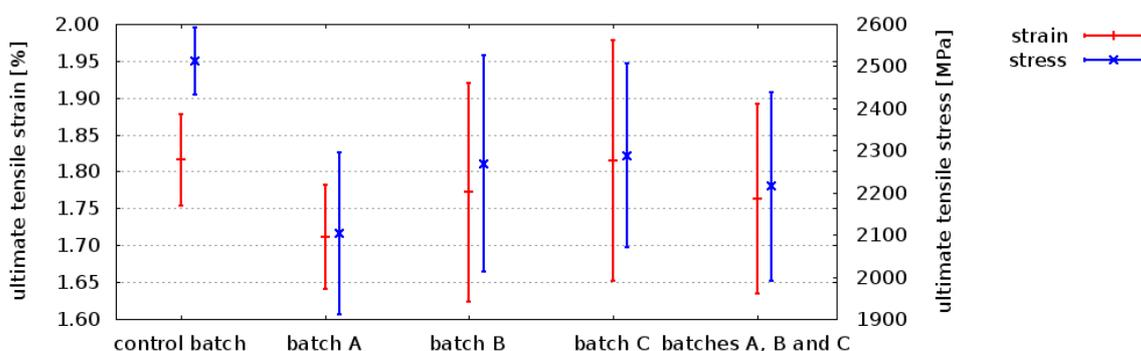
Figure 1: Uniaxial tensile tests conducted on unidirectional UD 0° flat samples [6]
