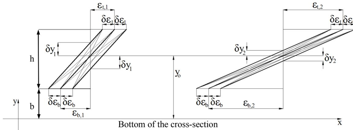
Figure 1: The magnitude of the strain measurement influences the uncertainty of the location of the neutral axis; the larger the strain magnitude the smaller the uncertainty. Figure modified from [1].
