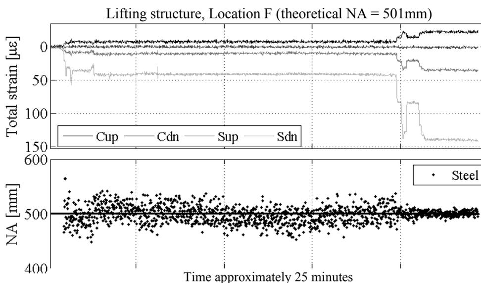
Figure 5. Strain at location F during the lifting from the floor onto supports. Cup is sensor at concrete up, Cdn is sensor at concrete down, Sup is sensor on the upper steel flange, and Sdn is sensor on the lower steel flange. The neutral axis location measured from the bottom of the cross-section as measured by the steel sensors.
