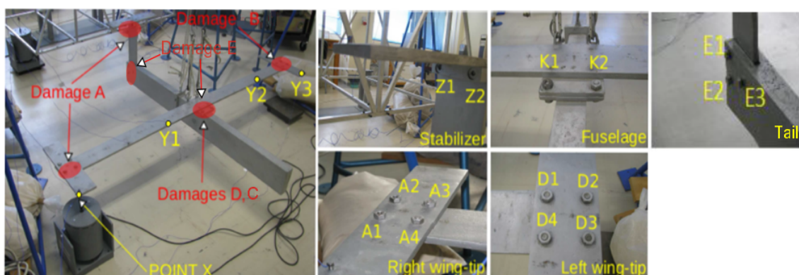
Figure 1 : The aircraft scale skeleton structure and the experimental set-up: The force excitation (Point X), the vibration measurement locations (Points Y1–Y3), and the bolts connecting the various elements of the structure.
