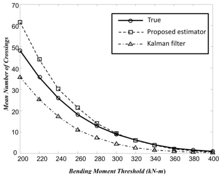
Figure5. Mean number of threshold crossings for the simulated system (“True”), the proposed model-based estimator and the KF.
