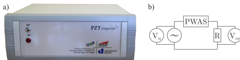
Figure 2: a) PZT Inspector, b) measurement circuit used for impedance measurements
