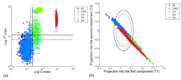
Figure 4: a) Q index vs.  $T^2$  index with damage thresholds for 95% and 99% of confidence (dashed line and solid line respectively). b) Projection into the two first principal components with damage thresholds for 95% and 99% of confidence (dashed line and solid line respectively).
