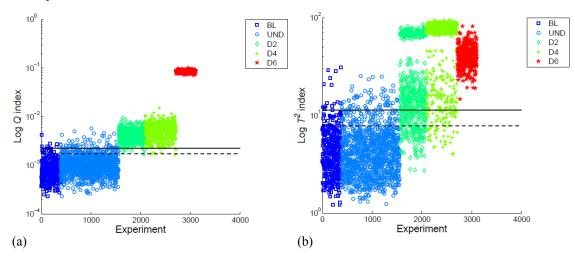
Figure 3: a) Q index with damage thresholds for 95% and 99% of confidence (dashed line and solid line respectively). b)  $T^2$  index with damage thresholds for 95% and 99% of confidence (dashed line and solid line respectively).
