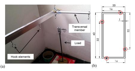
Figure 1: a) Aluminum beam. b) Location of FOS at cross section. Dimensions in mm.
