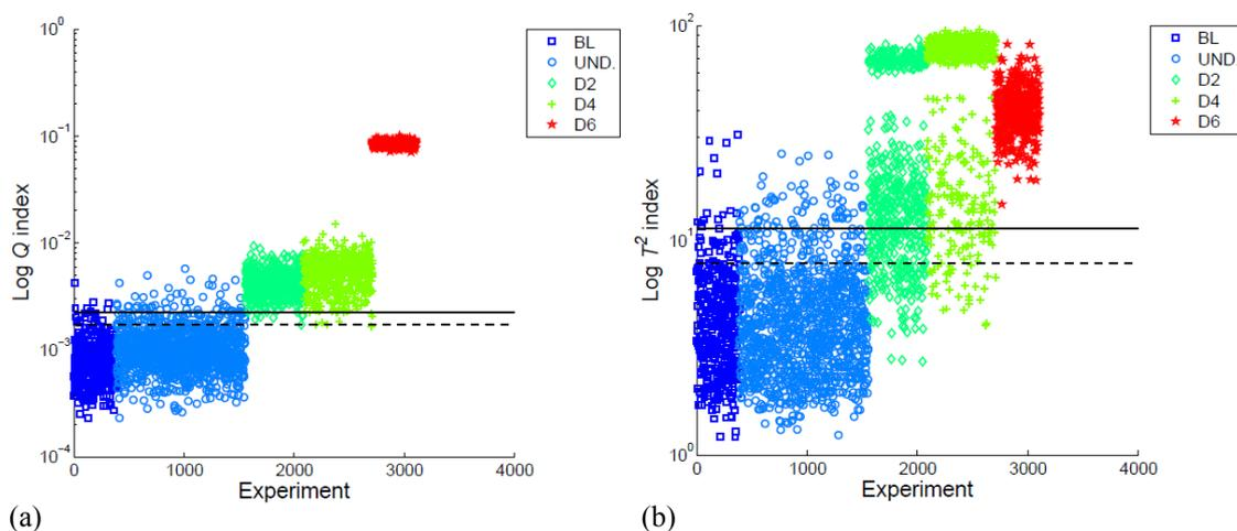
Figure 3: a)  $Q$  index with damage thresholds for 95% and 99% of confidence (dashed line and solid line respectively). b)  $T^2$  index with damage thresholds for 95% and 99% of confidence (dashed line and solid line respectively).
