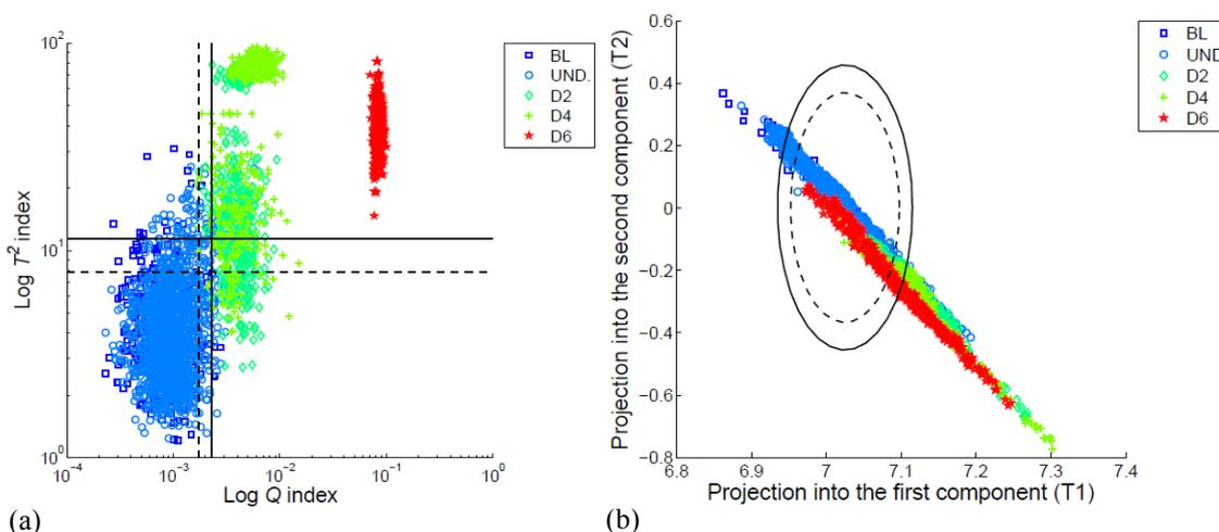
Figure 4: a)  $Q$  index vs.  $T^2$  index with damage thresholds for 95% and 99% of confidence (dashed line and solid line respectively). b) Projection into the two first principal components with damage thresholds for 95% and 99% of confidence (dashed line and solid line respectively).
