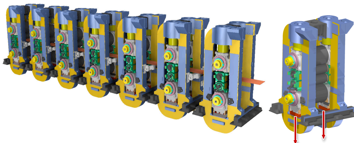
Figure 2: a) Seven stand finishing mill, b) Single stand with pressure cell
