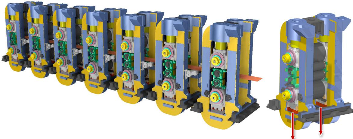
Figure 2: a) Seven stand finishing mill, b) Single stand with pressure cell
