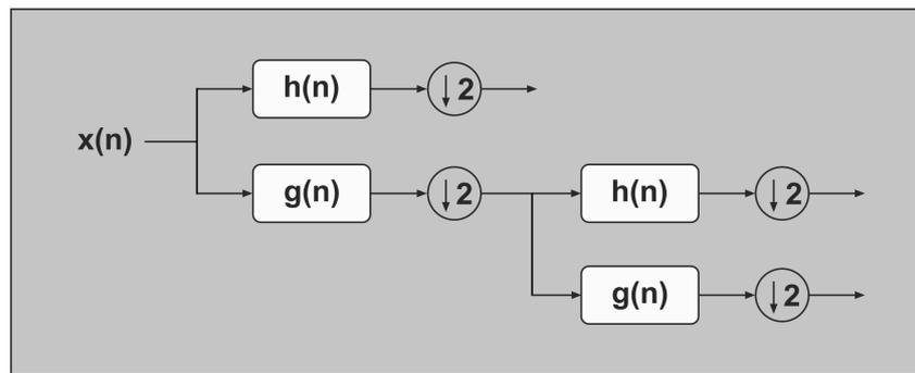
Figure 1: Filter belt of discrete wavelet transform
