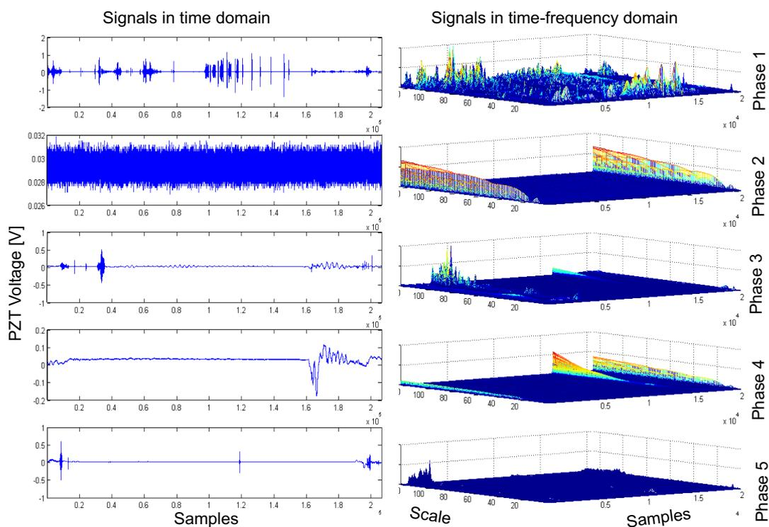
Figure 5 : Acoustic Emission signals and the corresponding CWT results during forward stroke
