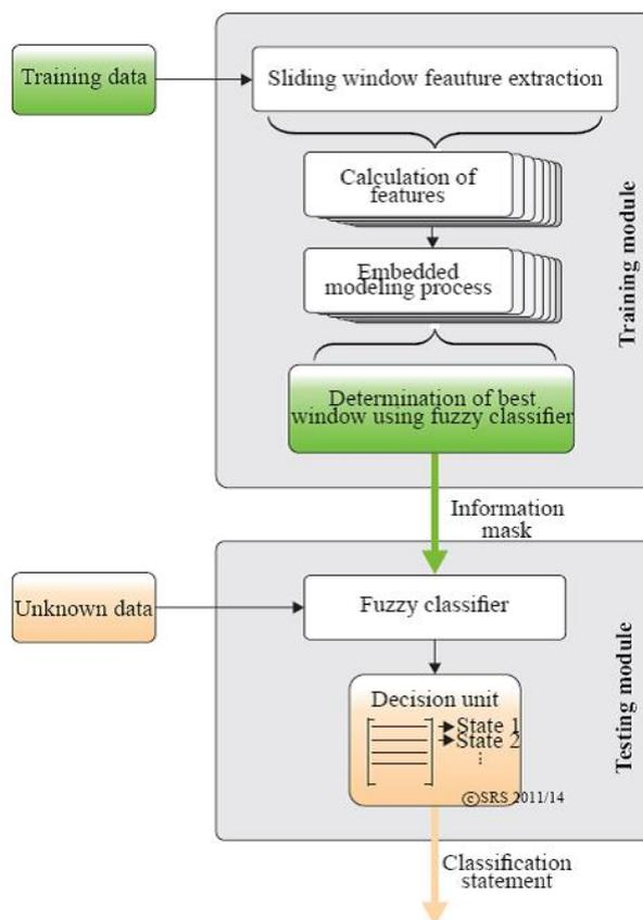
Figure 3 : Basic structure of AFFCA [13]
