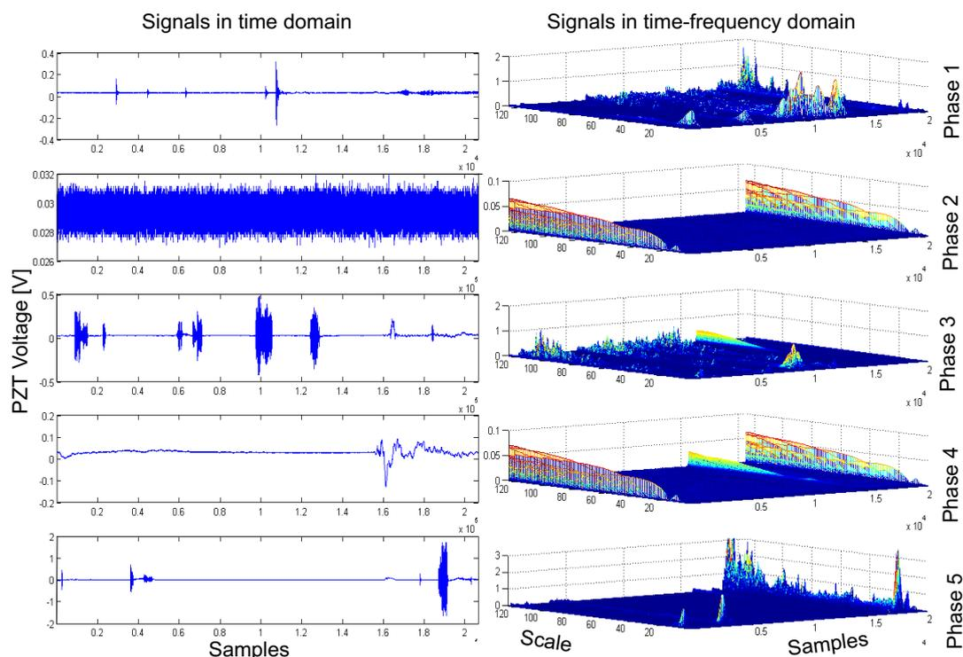
Figure 6 : Acoustic Emission signals and the corresponding CWT results during backward stroke
