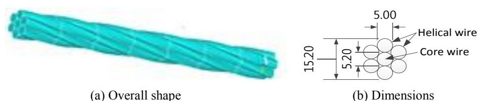
Figure 1: Structure of the considered 7-wire strand
