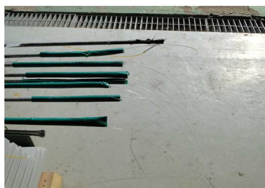
(b) Completed built-in optical fibre sensor specimens
