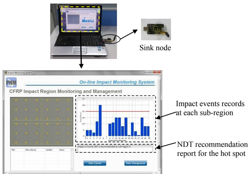
Figure 7: Evaluation system setup
