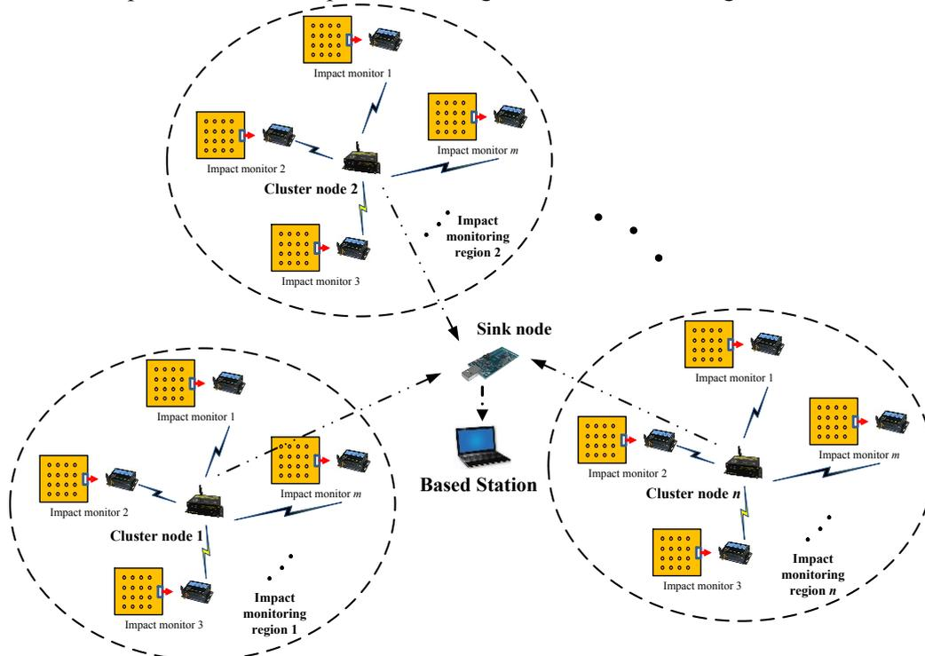
Figure 5: Illustration of the on-line wireless impact monitoring system
