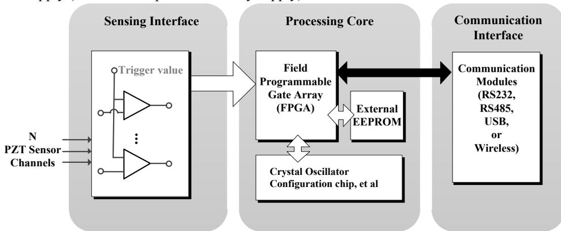
Figure 2: Architecture of the digital impact monitor
