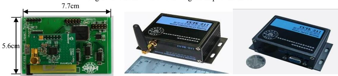
Figure 3: The miniaturized PZT-based impact monitors
