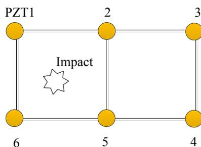
(a) Schematic layout of PZT sensors
