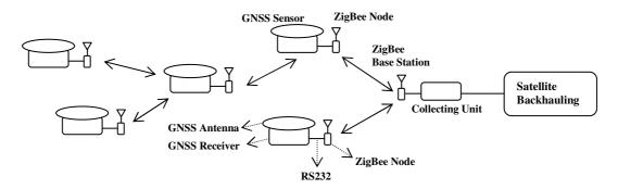
Figure 1: Wireless GNSS sensors network
