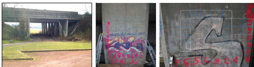
Figure 5 : On site test and example of identification of the measurement zones a) Structure b) Prior auscultation pattern c) Auscultation zones
