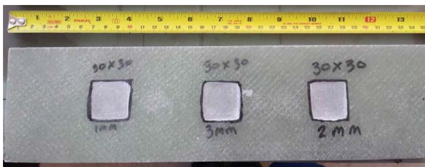
Figure 4: The bottom view of a piece of GFRP (8 mm thick) sample with three defects (30x30mm) measured 1 mm, 2 mm and 3 mm deep from the bottom.
