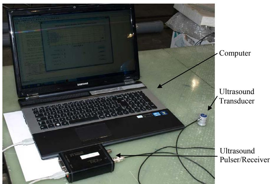
Figure 1: Ultrasonic NDT system.
