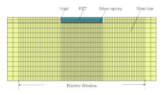
Figure 2:Mesh design of a steel rebar with PZTs (partial)
