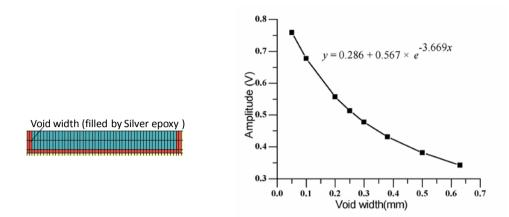
Figure 6:Parametric study of void width filled with silver epoxy
