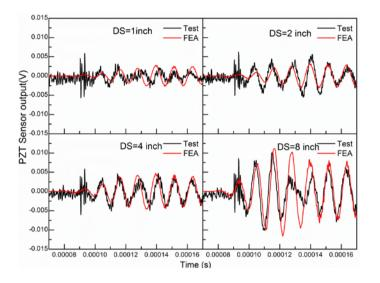
Figure 4:Sensor output from simulation and test for beam with debonding damage
