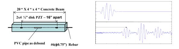
a) Layout of the PZT rebar concrete beam b) Test wave and the principle of SHM Figure 1:PZT based active sensing SHM system for concrete beam
