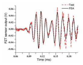
Figure 3:Sensor output from simulation and test for PZT steel rebar
