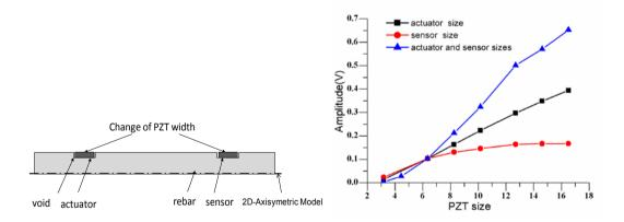
a)Layout of PZT size optimization b)Sensor output changes with different PZT sizes Figure 7:Signal optimization with PZT sizes
