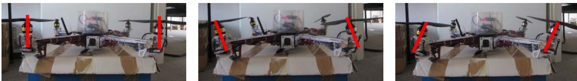
Figure 9: Vector thrust motor operating. Lines indicate the motor angle.
