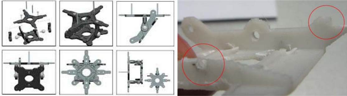
Figure 7 Left: Off the shelf vector thrust joint. Right: Weak contact points (circles)
