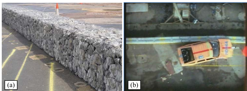
Figure 1: (a) Gabion barrier; (b) Concrete barrier crash test [9] .
