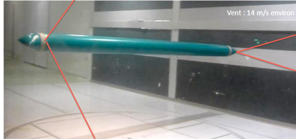
Figure 4 : The inflatable beam in the wind tunnel (average air velocity : 14 m/s). The four cables are colorized to highlight their location.
