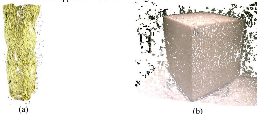
Figure 3: Stereo reconstruction of (a) synthetic data, and (b) concrete cube in an underwater setting
