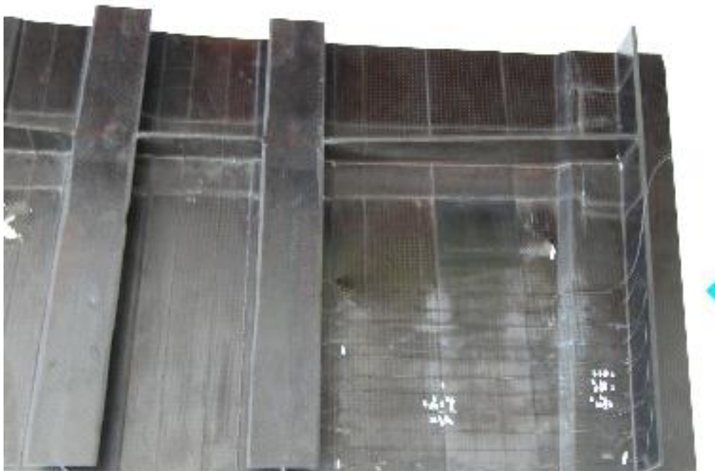
Figure 9 Cured CFRP structure, with bonded optical fibre
