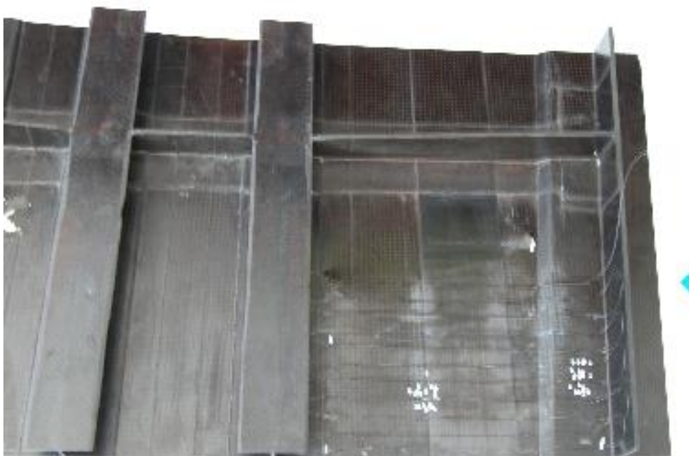
Figure 9 Cured CFRP structure, with bonded optical fibre
