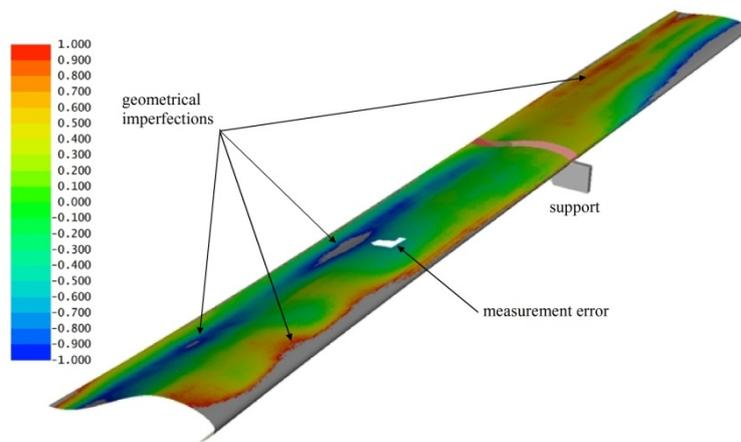
Figure 3: Measured geometrical imperfections on a rotor blade segment
