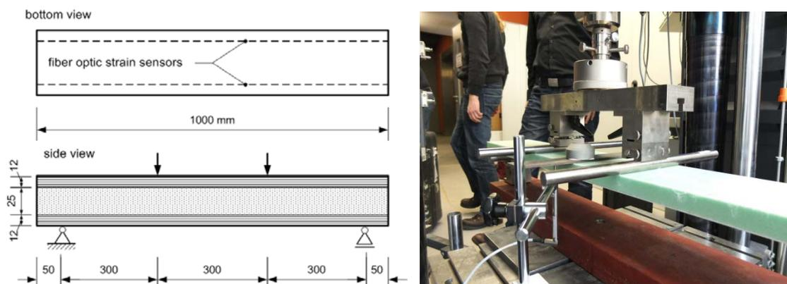
Figure 8: General test setup for sandwich plate
