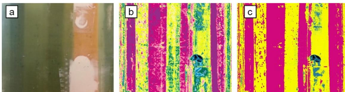
Figure 7: Results of ultrasonic scan on a rotor blade section; a) photo of the test section, b) ultrasonic scan with 64 colours, c) ultrasonic scan with only 5 colour grades giving a better position of manufacturing defects (e.g. voids in glue are red points in a yellow band)
