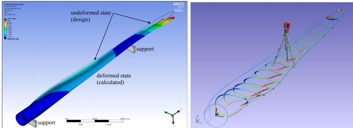
Figure 2: Comparison of design geometry and calculated deformed state under dead weight (left) and contour sections measured by laser tracker (right)
