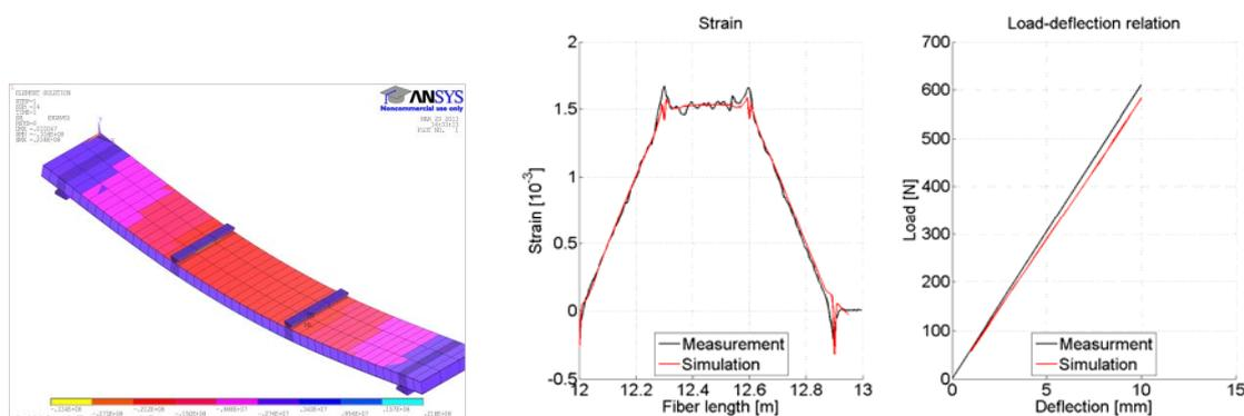
Figure 9: FE model (left); comparison of computational and experimental results (right)
