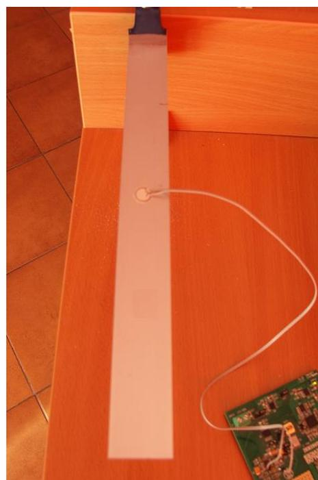
Figure 2: Object of investigations – aluminum alloy specimen.
