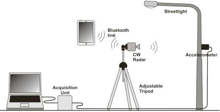
Figure 4: experimental setup for street light oscillation measurement
