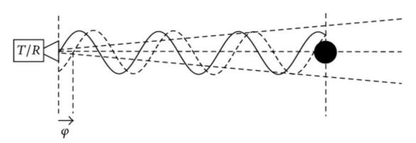
Figure 1: Working principle of interferometry
