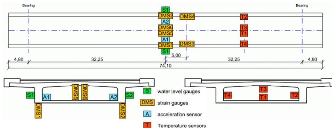
Figure 3: Monitoring system installed on Teufenbach Bridge
