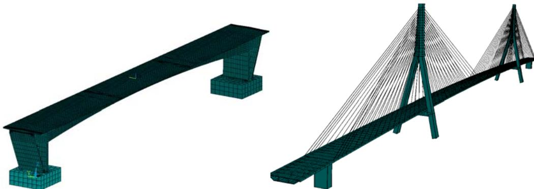
Figure 5: Finite-Element models. Left: Teufenbach Bridge, right: Guadiana River Bridge
