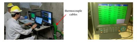
Figure 9: Remote measurement station to control the OBR-4600 (left) and TC measurement station (right)
