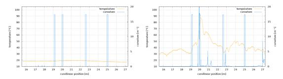
Figure 14: Distributed curvature measurements during the first day – initial state on left
