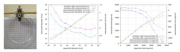
Figure 3: Curvature radius (centre) and strain measurements (right) with experimental set-up (left)
