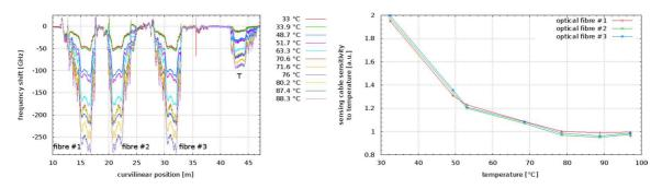
Figure 5: Temperature calibration measurements (left) and relative sensitivity  $\frac{\Delta v_{\{T\}_i}}{\Delta v_{\{T\}_{ref}}}$  results (right)
