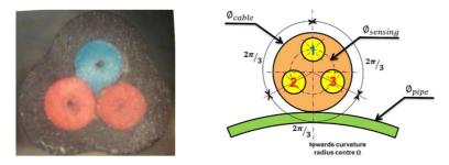
Figure 2: Strain sensing cable manufactured by Acome<sup>TM</sup>, devoted to curvature radius & strain measurements
