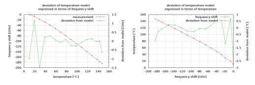
Figure 1: Temperature calibration results – Optical fibre in loose tube, free from friction effects
