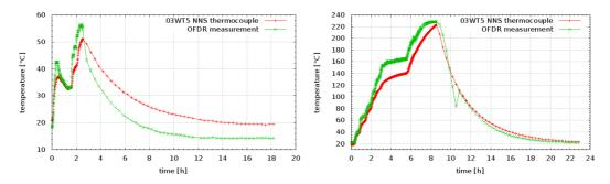
Figure 11: OFDR measurements compared with 03WT5 NNS thermocouple (left: 1st day, right: 2nd day)
