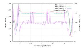
Figure 4: Strain measurements along bended instrumented pipe with experimental set-up on left
