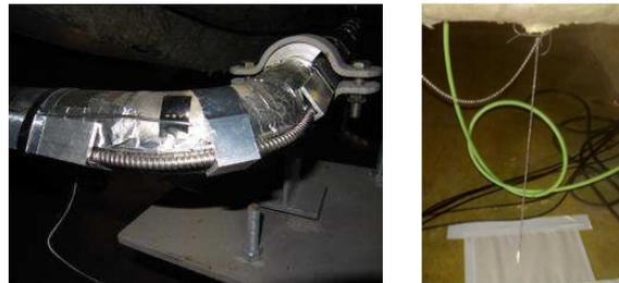
Figure 8: Thermocouple temperature sensor (left) and displacement sensor (right) for reference measurements
