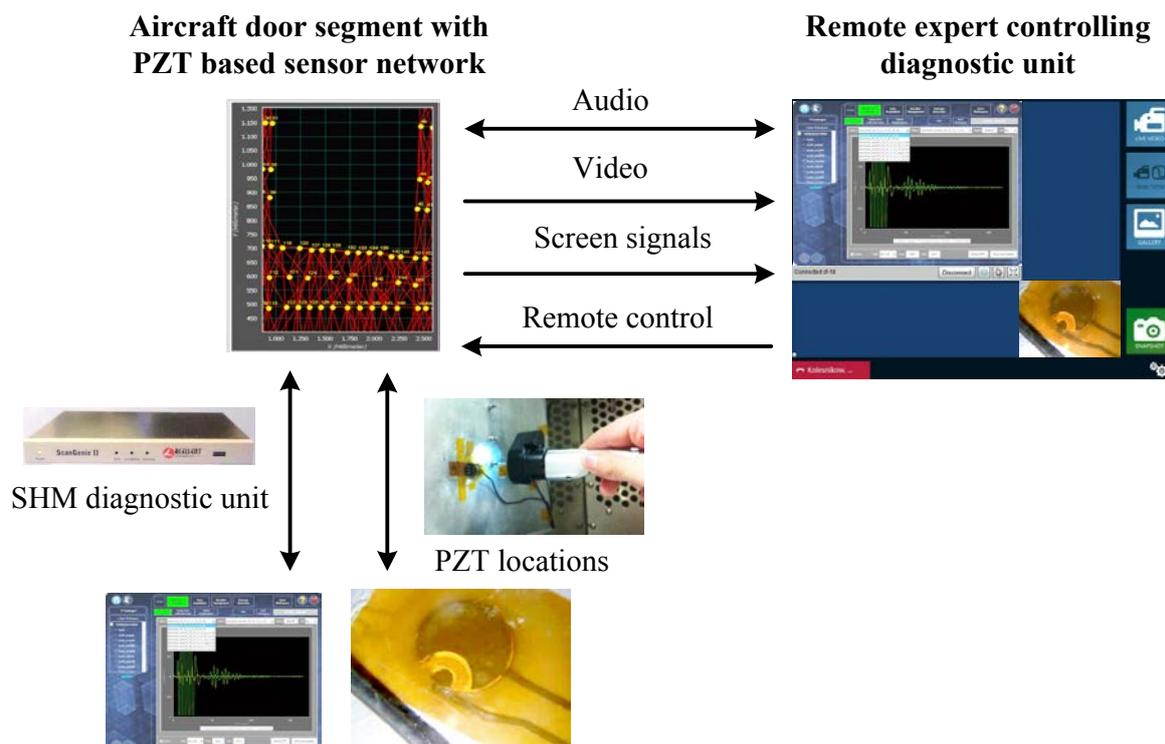
Figure 1: Using the OMA system for Remote SHM
