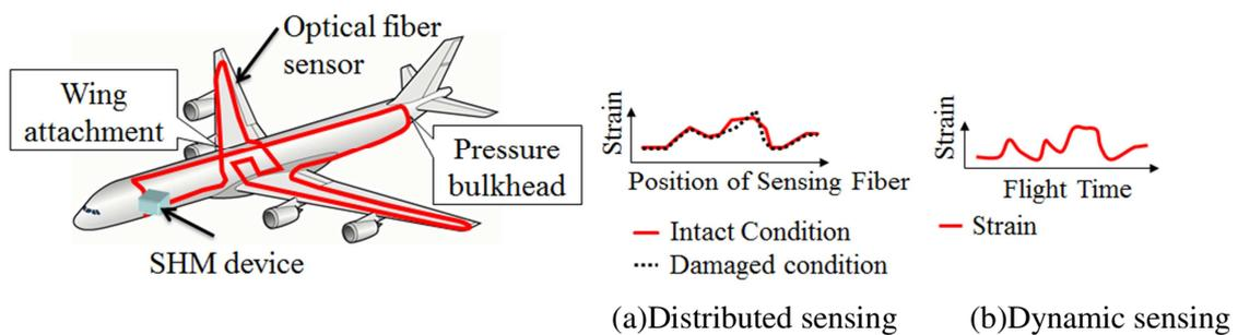
Figure 1: Application scenario of BOCDA-SHM system
