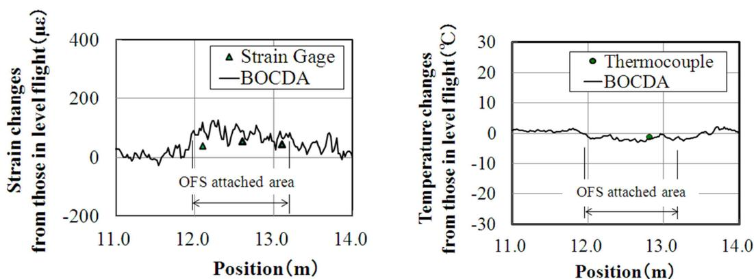
Figure 7: Distributed strain and temperature changes during steady banking flights
