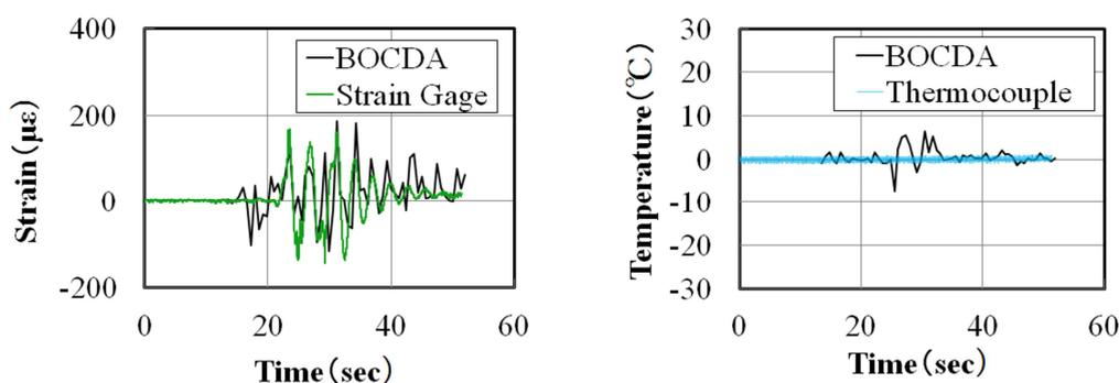
Figure 5: Dynamic strain and temperature changes during right-left turning flights
