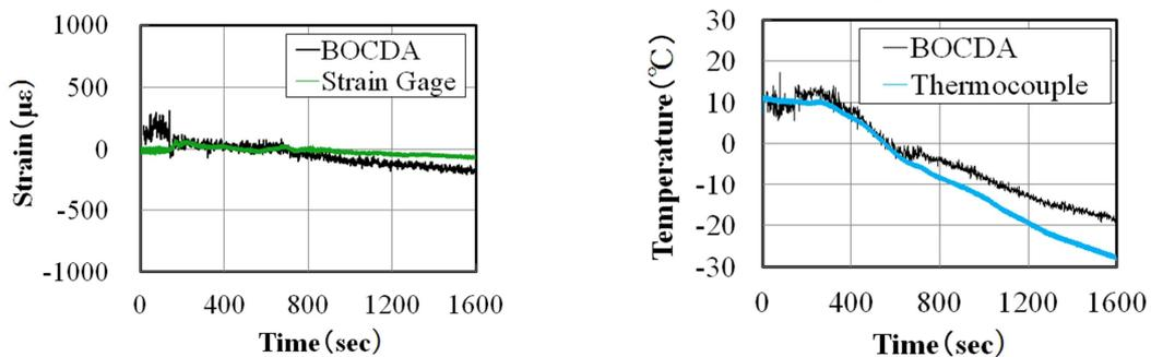
Figure 4: Dynamic strain and temperature changes during take-off and ascending
