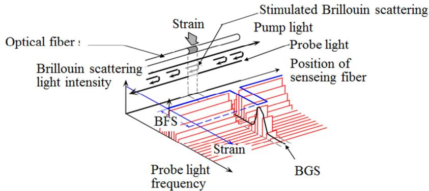
Figure 2: Measurement principle of BOCDA
