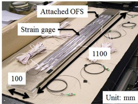
Figure 8: Test specimen
