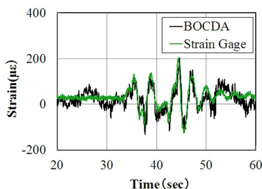
Figure 6: Dynamic strain changes during right-left turning flights
