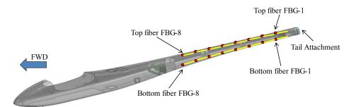
Figure 2: Boom general layout and the routing of the embedded optical fibers in the boom. 16 FBGs were located at points of interest (RHS boom shown. LHS is similar.)
