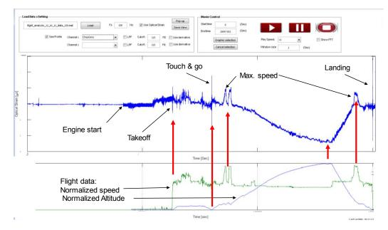
Figure 3: Flight data GUI; Typical Boom FBG readings during flight. Note the 'touch & go', maneuver and landing
