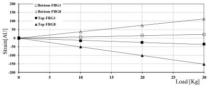
Figure 4: Typical Boom FBG calibration. At identical boom stations, top and bottom FBGs will have different strain magnitude
