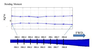
Figure 7: Boom bending moment envelope during landing
