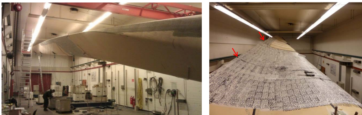
Figure 1: The 34m blade in the experimental Blade Test Facility at DTU Wind Energy. Left: Suction of blade. Right: Upper (pressure) side of blade. Accelerometers is marked with a red arrow
