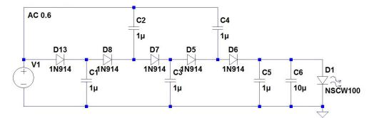
Figure 6. Voltage Multiplier Energy Harvesting Circuit.
