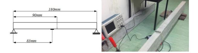
Figure 3. (a) Position of Energy Harvester and Damage Location (b) Experimental Setup
