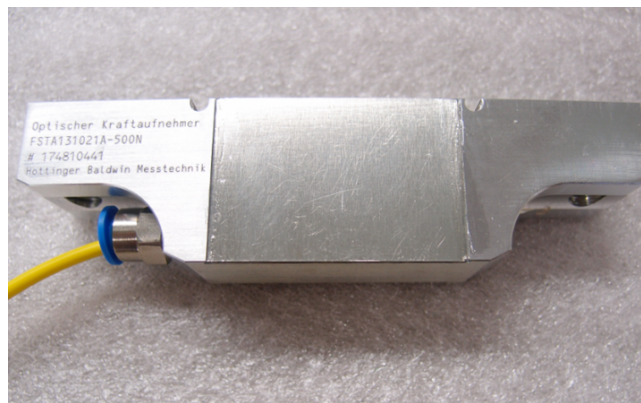
Figure 4 : Fibre Optic Force Sensor FSTA131021-500N
