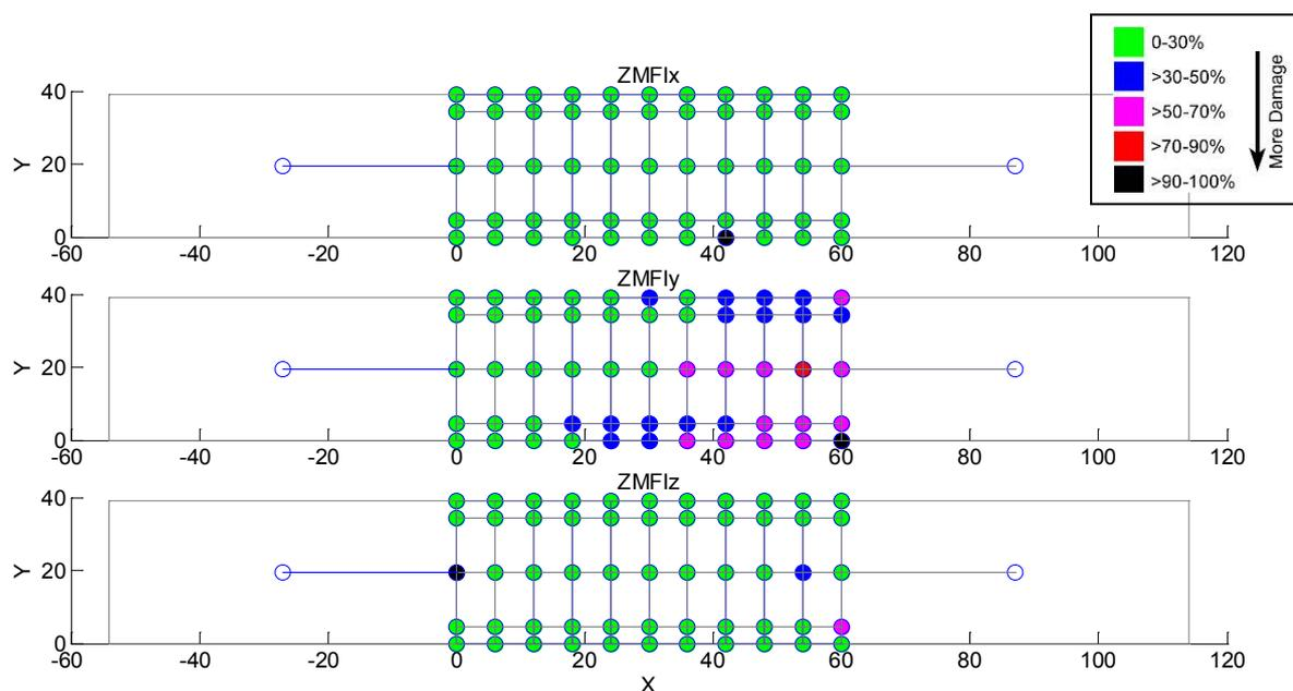
Figure 4: Normalized Modal Flexibility Index (ZMFI) results for each direction by location
