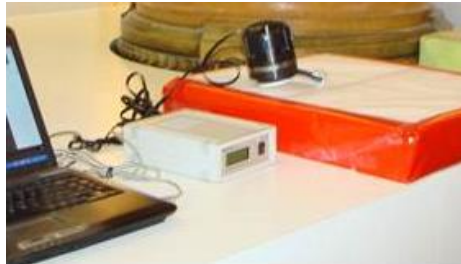
Figure 4: Holographic radar system Rascan 4/4000.
