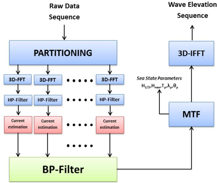
Figure 1 Block diagram of the inversion procedure
