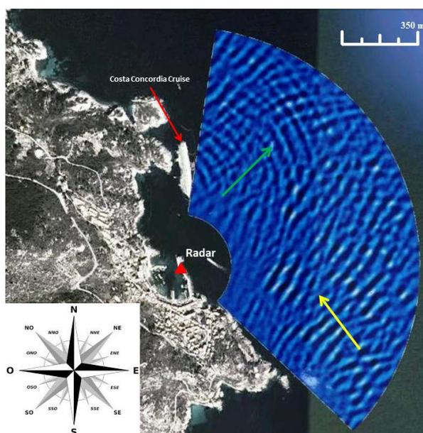
**Figure 5** Sea wave height reconstruction provided by the Remocean system. The yellow arrow indicates the direction of the dominant wave mode; the green arrow indicates the direction of the secondary wave mode.
