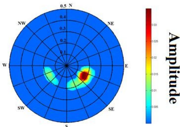
Figure 4 Directional Spectrum obtained by the Remocean system
