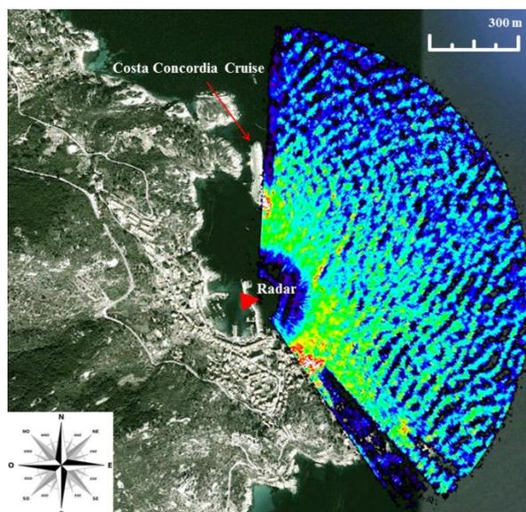
**Figure 3** A radar image collected during the storm. The position of the radar and the ship wreck is indicated by the red triangle and the red arrow, respectively.
