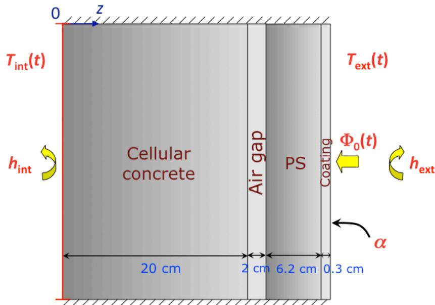
Figure 7: Schematic representation of the wall considered in the thermal modeling
