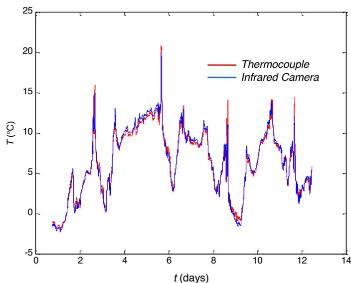
Figure 4: Comparison between thermocouple and corrected infrared measurements for the left upper zone of the western façade
