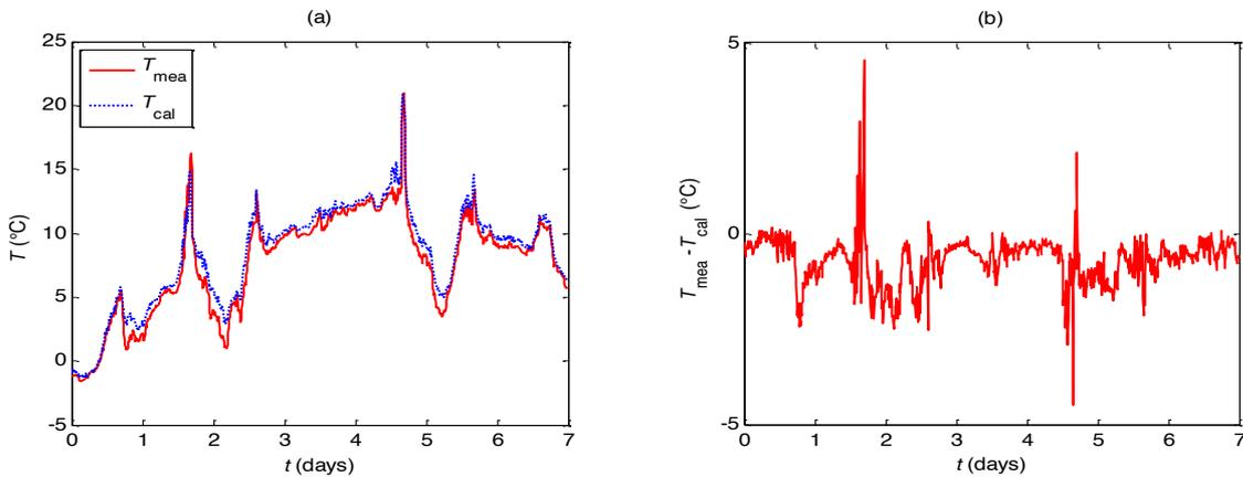
Figure 8: Exterior wall surface temperatures – first floor of the western façade
