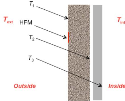
Figure 6: Schematic representation of the instrumentation used to measure the thermal resistance wall
