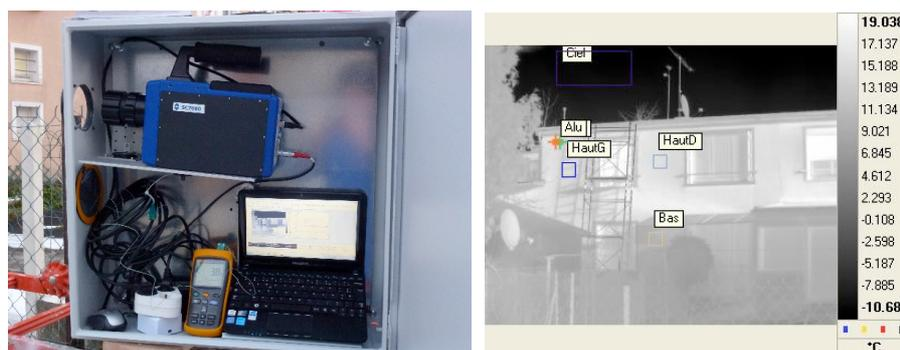
Figure 3: View of the thermographic instrumentation (left) and example of thermal image recorded during a sunny day (right)
