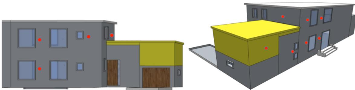
Figure 2: Views of the PANISSE platform; eastern and northern façades (left), northern and western façades (right); red points indicate the positions of thermocouples
