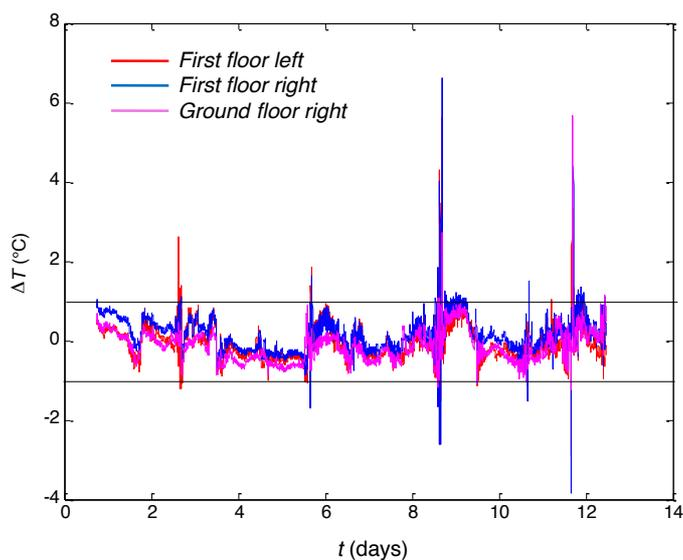
Figure 5: Temperature differences between thermocouple and corrected infrared measurements for three zones of the western façade
