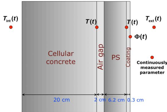
Figure 1: Schematic description of the PANISSE walls structure
