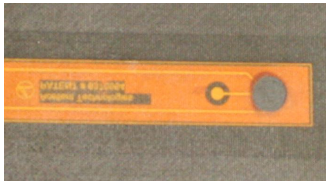
Figure 5: Co-Bonded Smart Layer® after PZT transducer disc removal
