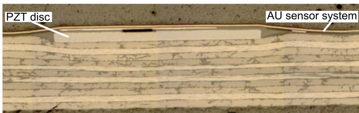
Figure 1: Micrograph of fiber misalignments underneath a PZT of an AU sensor system (Acellent Smart Layer®)
