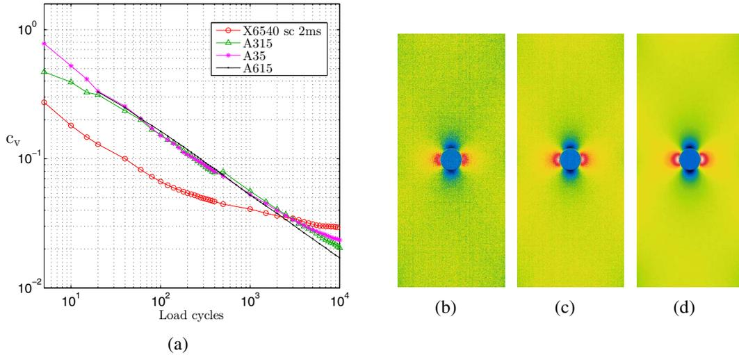
Figure 1: Graph (a) shows signal noise (expressed as the coefficient of variation  $c_v$ ) as a function of correlation length for a photon detector (FLIR X6540 sc) and 3 microbolometers (FLIR-A35, A315 and A615). Thermoelastic scans (b)-(d) are from an A615 after 100, 1000 and 10000 load cycles respectively.
